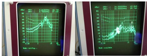
High Frequency Noise Generated by VFD Above requested standard limits
